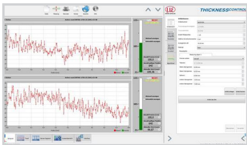
Point cloud diagrams of two laser line sensors
